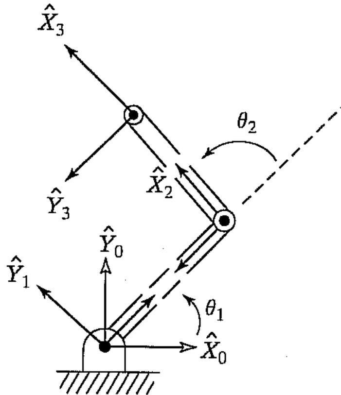
FIGURE 5.9: Frame assignments for the two-link manipulator.
