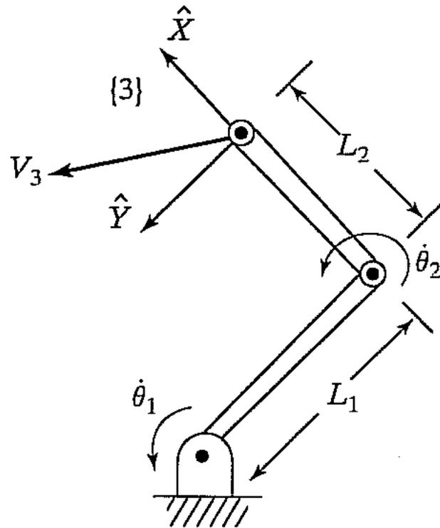
FIGURE 5.8: A two-link manipulator.
