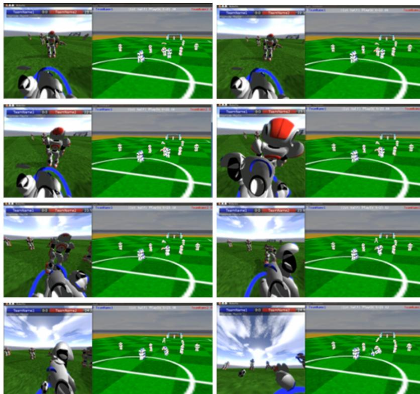
**Fig. 1.** Pictures from local(left) and global(right) vision Systems. In a zigzag way from the left top screen shot to the right bottom one, they are snapshots of collision between two robots. The last picture was taken as the robot was falling backwards and most of the visual information is from the sky.
