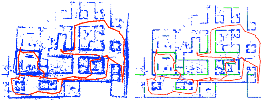
Fig. 2 Mapping with odometry (a) and mapping with proposed method (b)
