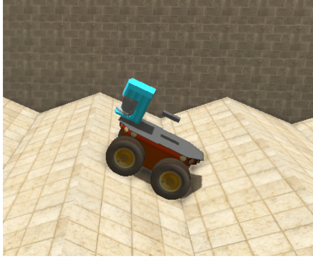
Fig. 1. This figure shows uneven floor consisted from prisms and a robot P3AT. The P3AT can run over prisms easily in this combination the size of the robot and the prism.
