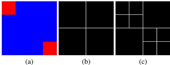
Figure 2: Quadtree segmentation: a) Image sample; b) First slice throughout entire image; c) Second slice only in specific blocks that satisfy the segmentation criteria.
