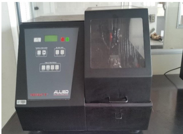
Figura 10: (a) Cortadeira automática TECHCUT 5 ™ , da Allied High Tech Products Inc. ® e (b) prensa de embutimento TECHPRESS 2 ™ da Allied High Tech Products Inc. ® .
