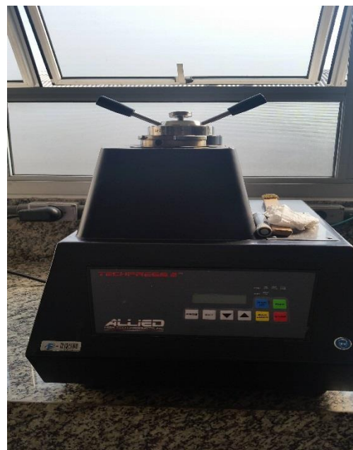
Figura 10: (a) Cortadeira automática TECHCUT 5 ™ , da Allied High Tech Products Inc. ® e (b) prensa de embutimento TECHPRESS 2 ™ da Allied High Tech Products Inc. ® .
