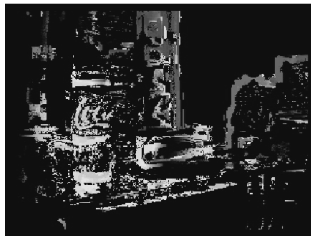
Figure 9. Disparity map generated from the 6 correspondences found in Figures 7a and 7b.
