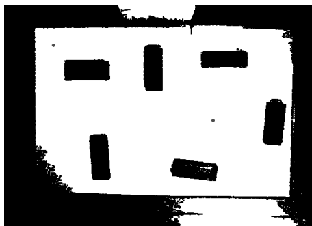
Figure 4. Output of the image processing level overlapped with the initial and final position markers.
