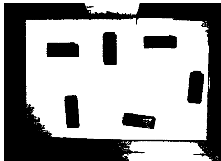
Figure 3. Detection of the obstacles by the image processing level, extracted directly from Fig. 2-c.
