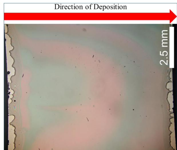
Fig. 1. Image of sample 10, measuring 10mm x 10mm, deposited with AZ5214E
