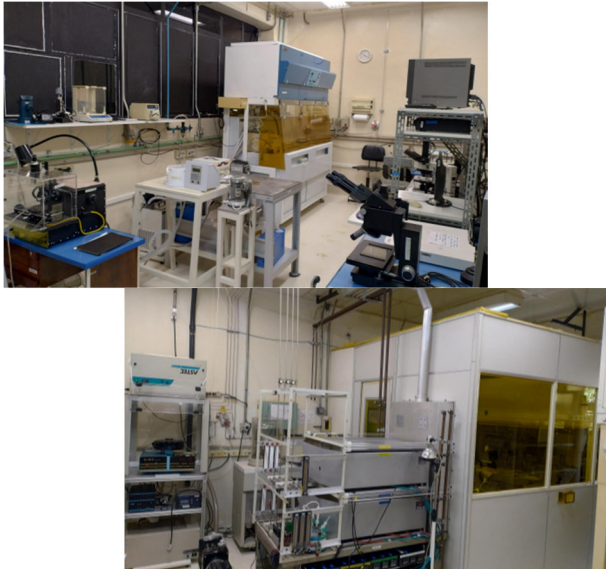
Fig.2. MIMEC overview; TOP: KOH chemical wet bench and diamond wheel dicer; BOTTOM; March plasma etcher, oxidation furnaces and litho area.
