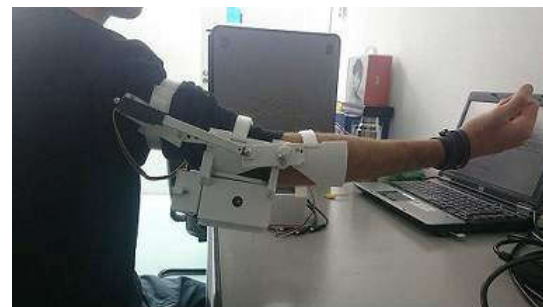
Figure 3 - PWM controlled arm orthosis for flexion movement.
