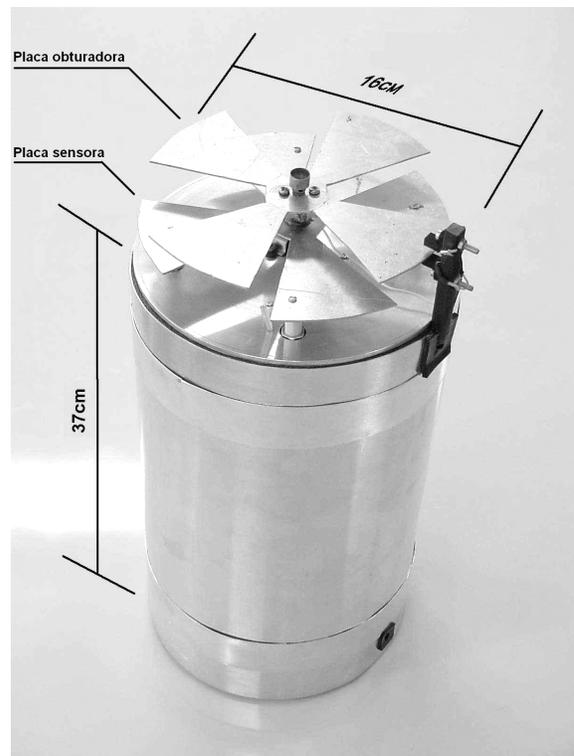
Fig. 3 - View of the field mill prototype.
