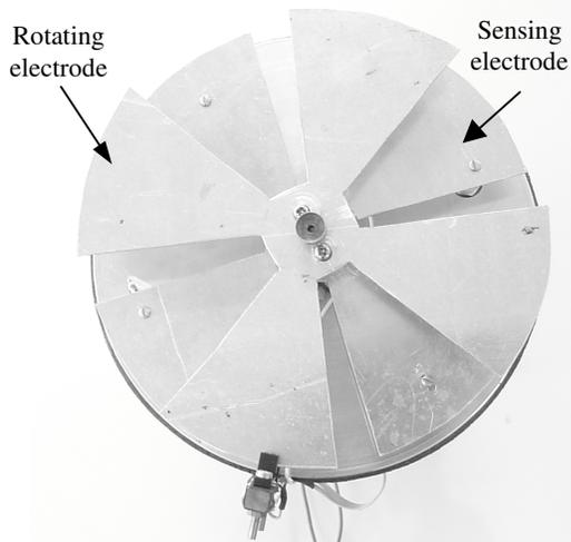
Fig. 4 - Construction details of the sensor electrode ( top of the field mill prototype ).
