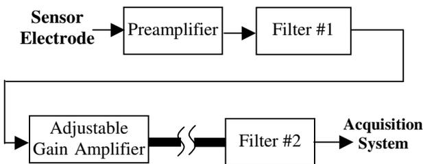
Fig. 5 - Electronics block diagram of the field mill prototype.
