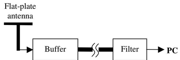
Fig. 6 - Electronics block diagram of the Flat-plate sensor.
