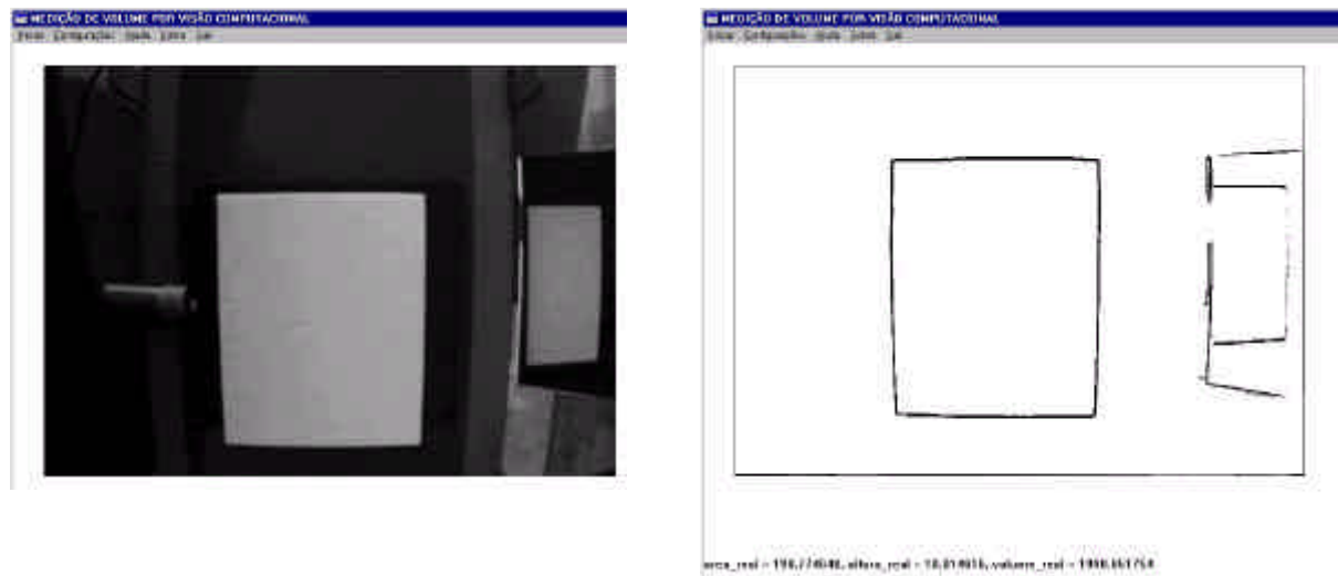
Fig. 5. An image from the camera and the corresponding edges.
