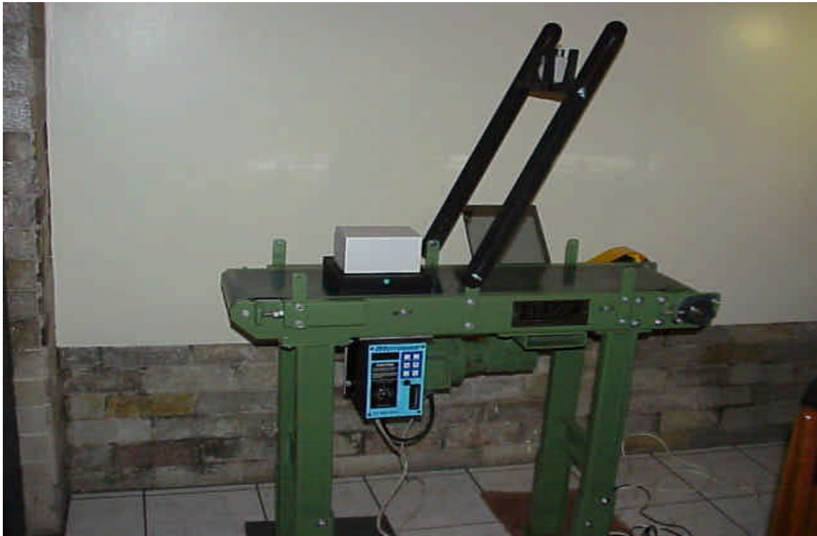
Fig. 4. The experimental setup, showing conveyor belt, camera, mirror and object.
