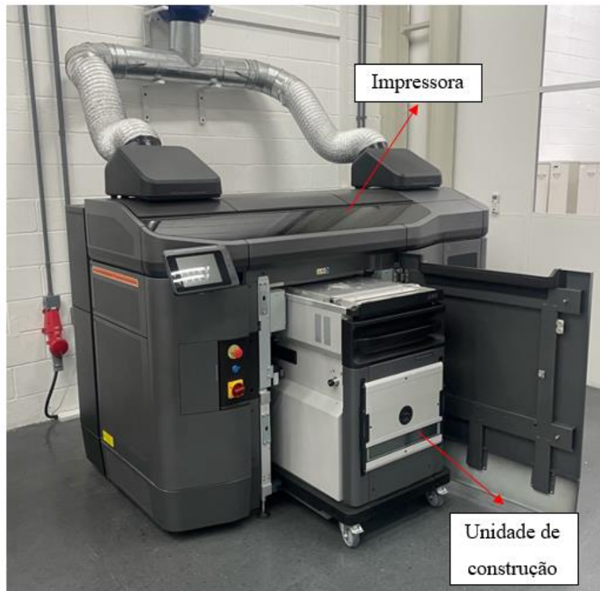
Figura 16 - Impressora 3D HP 4200 Jet Fusion
